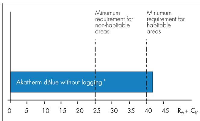
\* required  $R_w+C_{tr}$  40 results are extrapolated based on the  $R_w+C_{tr}$  25 results.
